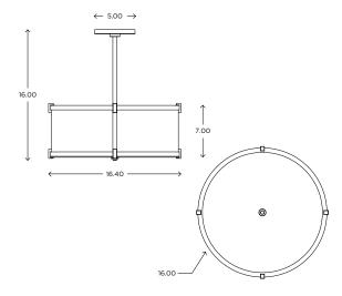
The Litebox combines subtle elements of classical style with a respect for contemporary simplicity. The result is a fixture that complements almost any architectural space. It is available in custom sizes, levels of trim (with or without crossbars), as a flush mount or pendant, and with custom finishes, diffusers, and lamping.
