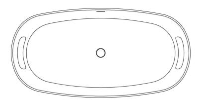
OVERFLOW IS INTEGRAL TO THE TUB
