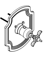
RAVEN 1/2" Thermostatic Mixer Valve with Stops Model: 4MRBRVC XX-XX
