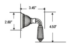
Flow Rate: 11 GPM@60PSI
