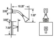
Flow Rate: 5.8GPM@50PSI
