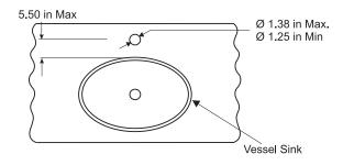
For marble (or similar material) deck, cut in the hole accordingly to the distances indicated in the figure.
