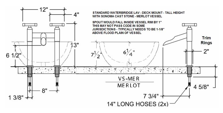
Please check with your local plumbing codes for the clearance required between the spout and the vessel sink.
